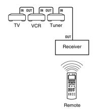
The remote sensor on this unit receives remote codes the same way as the remote sensor on the CTRL S IN component. This is useful if you place the other component away from this unit.
